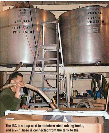
liner's filling valve. A volumetric pump fills the IBC.
